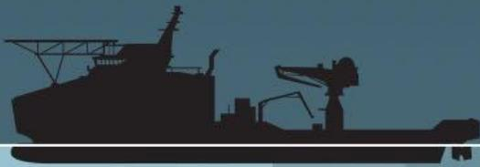
**22 feet** – the draft of the Australian offshore support vessel Ocean Shield, now searching for the black box. It is 347 long.
